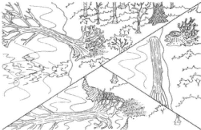
**Problem trees can be lopped. Leave roots in the ground and align the trunk against the bank toe to help stability. Trim the crown to reduce debris build-up during floods**
