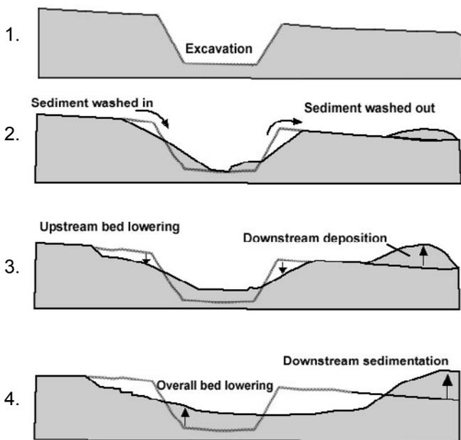
**Excessive sand and gravel extraction can trigger bed lowering and subsequent bank erosion**
