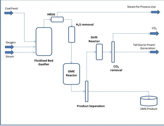
Figure 5, Pilot Plant Flow Diagram
