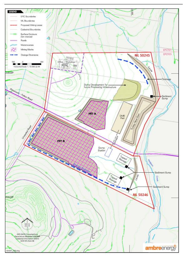
Figure 4, Demonstration Stage Mine and Infrastructure layout plan
