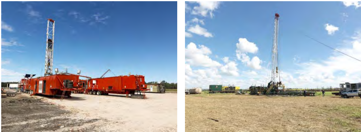
Figure 1-1 Typical CSG drilling rig and workover rig
