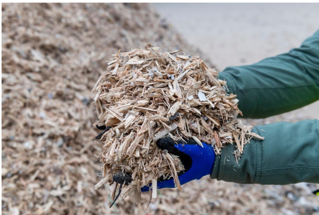
Processed engineered fuel produced to customer specifications including calorific value. Image courtesy of ResourceCo.
