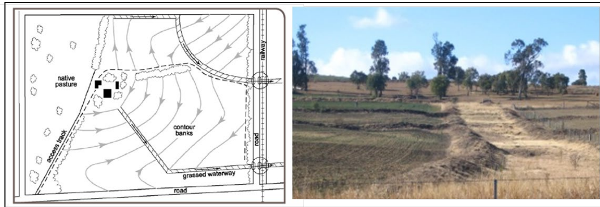
Figure 6: Left: Example of contour bank layout (Source: Figure 7.1, Chapter 7 Soil Conservation Guidelines). Right: Example of well-maintained contour banks on a Queensland farm (Source: https://www.qld.gov.au/environment/land/management/soil/erosion/management ).
