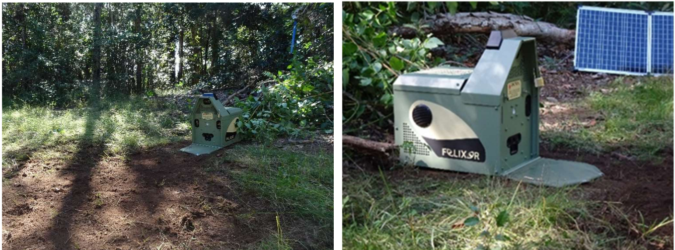
Figure 13: A Felixer device deployed to control feral cats in vine forest in Oakview NP.
